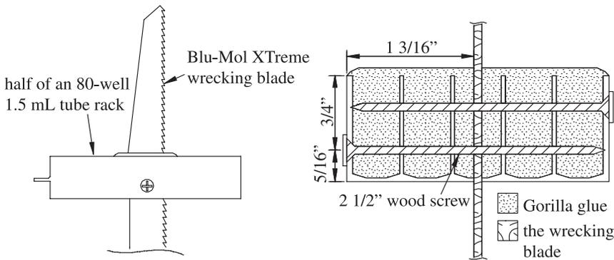
**Fig. 1** A diagram showing the modification of a tube rack for attachment to the reciprocating saw.
