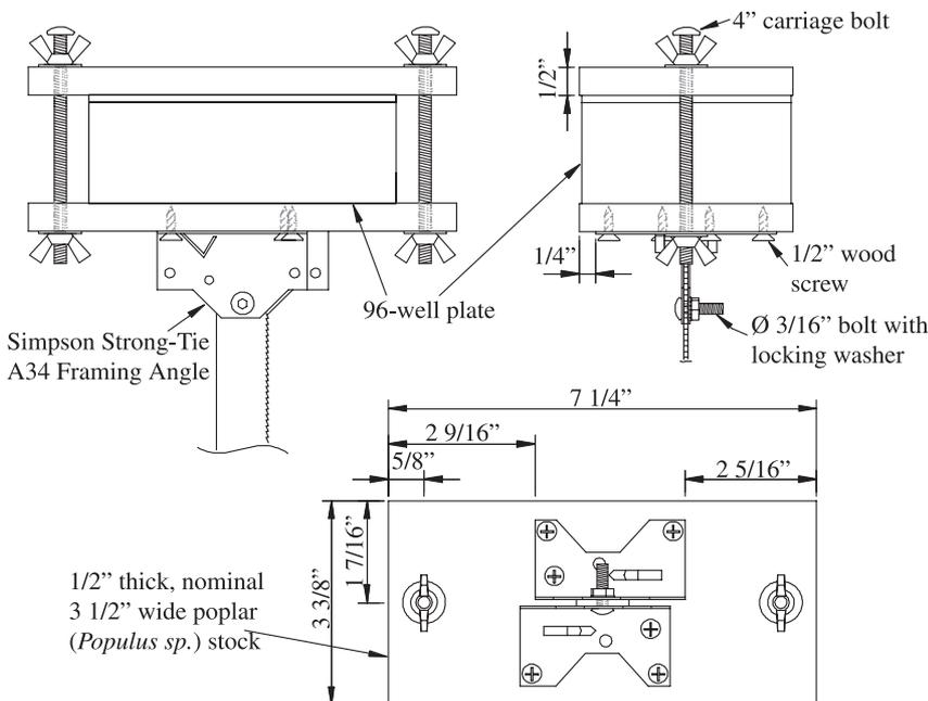
**Fig. 2** A diagram showing an adapter to hold a 96-well plate attached to the reciprocating saw.
